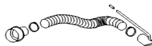
Step 2 Assemble remote pickup by slipping band clamp over remote hose, slide nozzle into end of hose, and secure with the band clamp. Connect reducer (or splice depending on remote) in the same manner.
