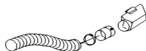
Step 1 Remove deck chute from the end of the vacuum's intake hose. Slip quick connect inside hose and secure with band clamp.
