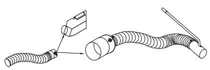
Switching from chute to remote is as easy as flipping the latch on the quick disconnect. Your Remote Pick Up Attachment will extend approximately 20 feet from your sweeper. Keep your hose as straight as possible for best results.
