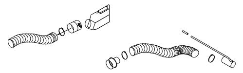
Step 1. Remove deck chute from the end of the vacuums intake hose. Slip quick connect inside hose and secure with band clamp.
